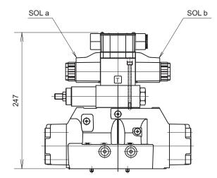
MT-02W-60 With MG-02P-1-60-%02 (type G, GR) (Hexagon socket head cap bolts used: M5 × 125, 4 pcs.)
